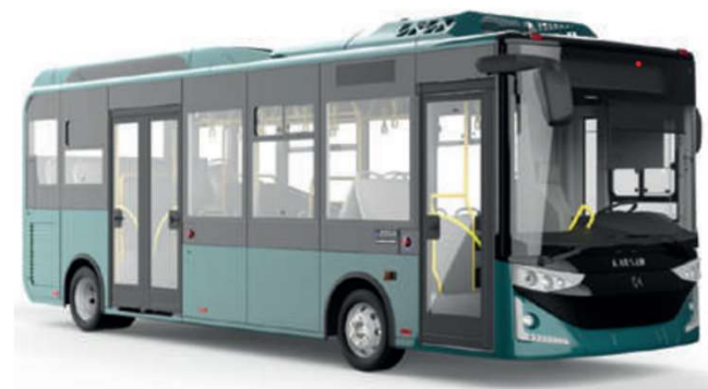
KARSAN ATAK – L 8,3m x L 2,4m x H 3,09m Autonomie 300 Km - 34 places debout
