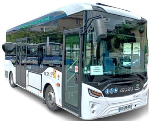
ISUZU NOVOCITI VOLT – L 7,9m x L 2,4m x H 3,2m Autonomie 350 Km - 22 places debout
